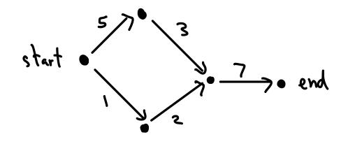
The maximum flow is the largest amount of water that can flow through this graph
