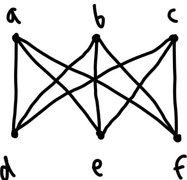
Pf: Suppose  $K_{3,3}$  has a planar representation. Then the induced subgraph formed by  $a, b, d, e$  is  $C_4$ :
