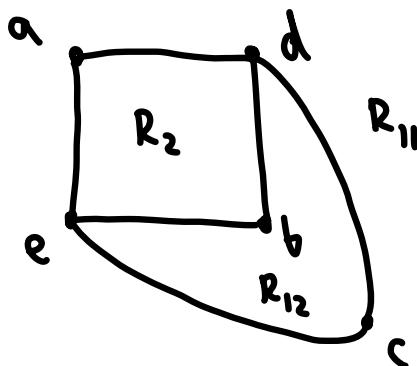
Finally, we need to place f and connect it to a, b, and c. To do so w/out edge crossings, f must lie in a region w/ a, b, c on the boundary.
